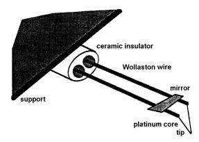
Fig. 2. Thermal probe (schematic).
