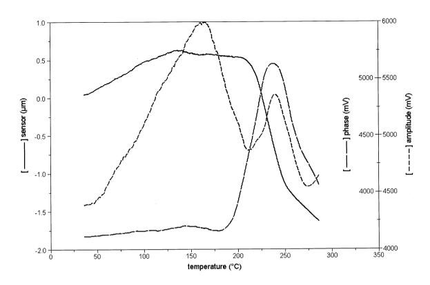
Fig. 9. Localised DMA of nylon showing the glass transition at 140°C and melting at 230°C.
