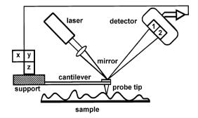
Fig. 1. Atomic force microscope (schematic).
