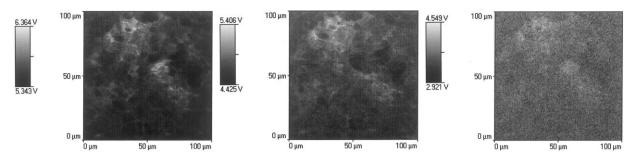
Fig. 4. AC thermal images of the voltage required to modulate the probe temperature with an amplitude of 5°C at 10 kHz (left), 30 kHz (middle) and 100 kHz (right).
