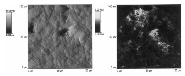
Fig. 3. Topographic (left) and DC thermal (right) images of the surface of a paracetamol tablet.
