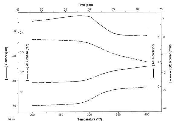
Fig. 6. Typical raw localised thermal analysis data for the melting of a polymer.
