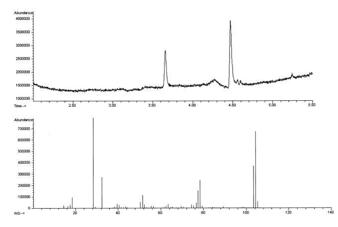
Fig. 11. Total ion chromatogram (top) from the pyrolysis of polystyrene. The peak at retention time 3.66 min is due to bleed from the GC column. The peak at 4.47 min is identified as styrene monomer (mass spectrum shown beneath) arising from the thermal degradation of the polymer.
