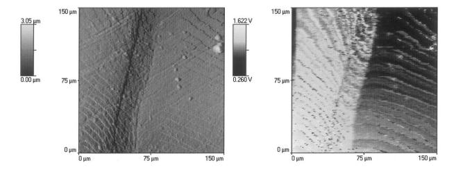
Fig. 10. Topographic (left) and thermal expansion (right) images of a polymer/metal interface. The polymer exhibits a higher thermal expansivity than the metal and shows up bright in thermal expansion image.
