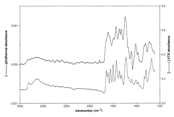
Fig. 12. Photothermal absorption spectrum of paracetamol (solid line) acquired using the thermal probe—the conventional ATR spectrum is shown (broken line) for comparison.
