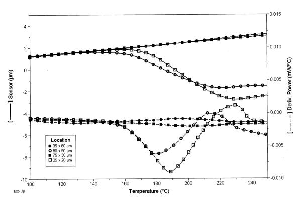
Fig. 8. Localised TMA (solid line) and DTA (broken line) curves for four different points on the images shown in Figs. 3-5.
